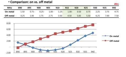
•GENERAL reads shorter by 40% or less off metal (or on non metal surface). With still reading 2.0 meters off metal, It can be applied for BOTH metal and off metal application.
