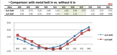
•GENERAL reads almost same, regardless of whether it is fastened with metal bolt in two holes (located on diagonal direction) or not. Stainless steel M3 bolt with round head is best fit for GENERAL.
